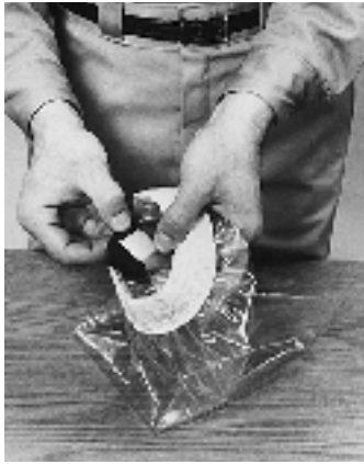
FIGURE 8 Removing inner Disperser part from Hood
