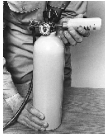
FIGURE 10 Leak Detection Check
