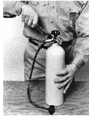
FIGURE 9 Removing Pressure Reducing Valve
